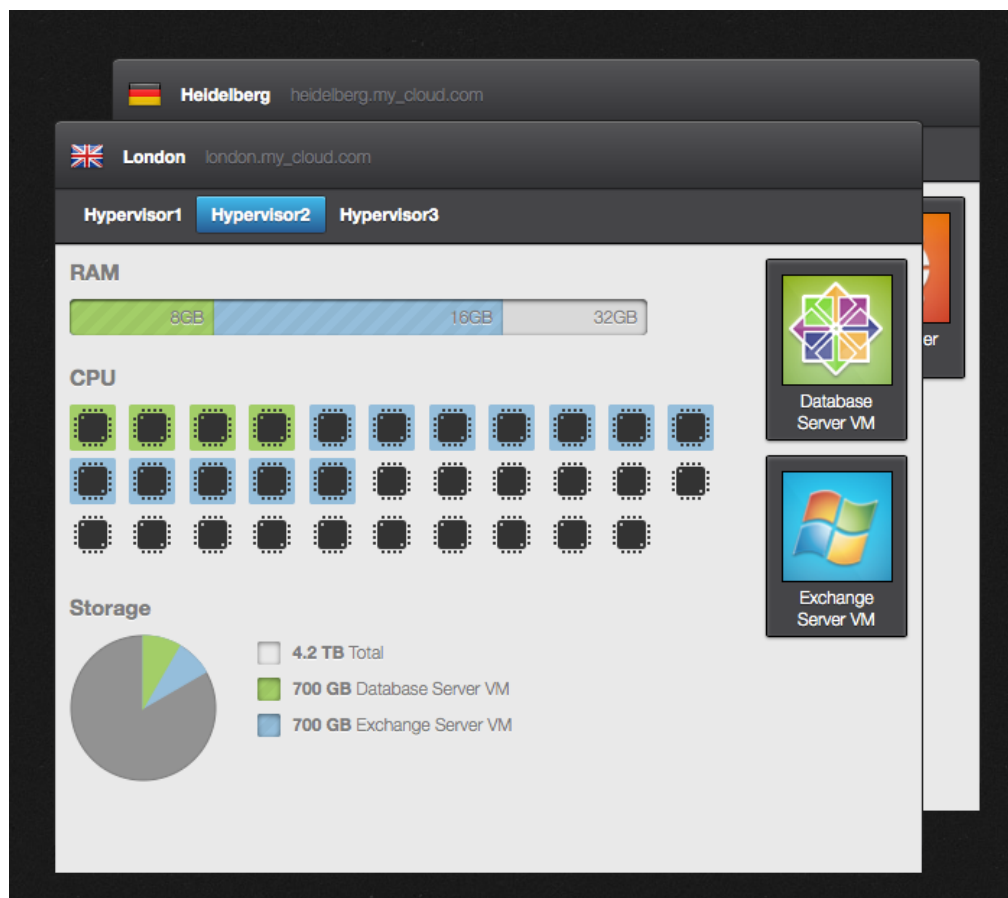
Figure 3.15: One hypervisor can support multiple VMs with different templates
