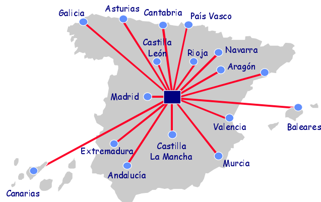
Figure 1. Topology of the RedIris IP/ATM backbone
