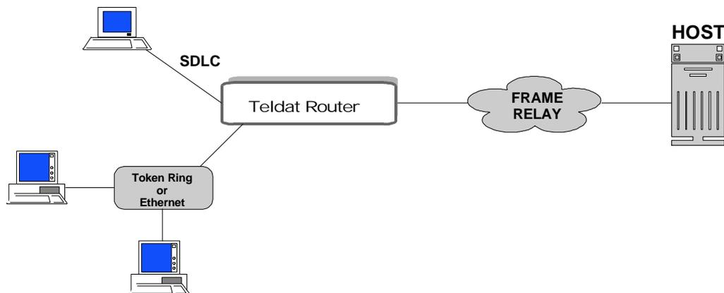
Through the **Teldat Router**, the end stations work in the same way they would if they were directly connected to the Host through the Token Ring network, Ethernet network, or through SDLC links. The Frame Relay network from this point of view, is totally transparent.
