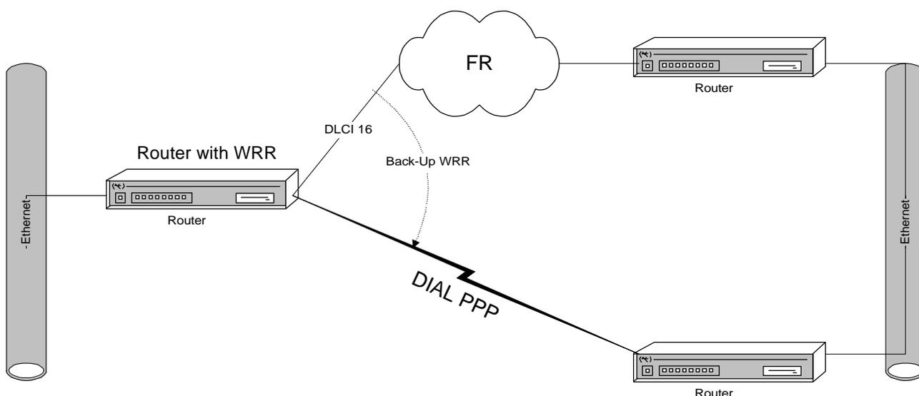
Supposing you wish to establish backup through WRR as indicated in the figure; when the Frame Relay DLCI 16 interface goes down, the Dial-PPP link activates establishing the call etc., until the DLCI recovers. The backup call is then released deactivating the Dial PPP link.
