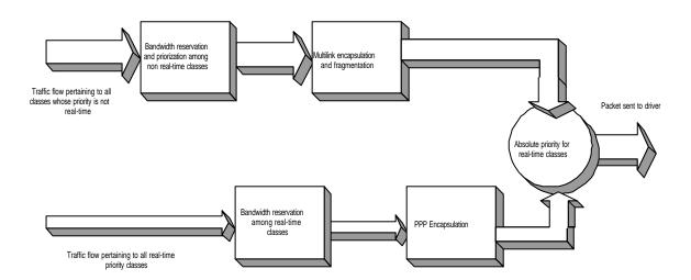
This scheme is contrasted with the generic scheme used for the rest of the encapsulations as, for example, Frame Relay where the process is as follows:
