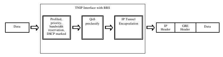
You can also see here that the *qos-preclasify* option is applied **after** the packet has been marked with a DSCP value. You must take this into account if BRS in the tunnel output interface is also applied.
