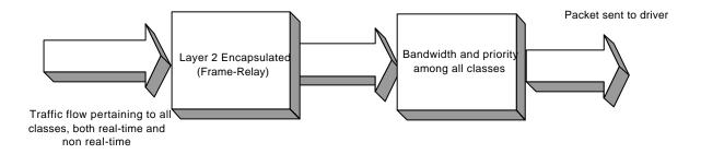
In cases of MP, the generic scheme is not valid as the MP assigns a sequence number to each packet. This number is used at the reception end to reorder them thus avoiding the possible disorder that can occur when using various links. The problem arises if BRS is placed after encapsulation in MP. Consequently after a sequence number has been assigned to the packets these become so disordered that in the majority of cases the end MP is incapable of reordering them and they are dropped.
