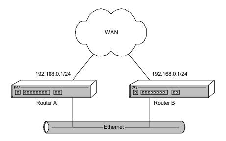
In this case, both Router A and Router B access the WAN with the same IP address (192.168.0.1) and we do not want the said network to be broadcast by RIP to the segment.
