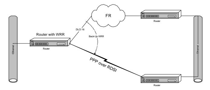
Supposing you wish to establish backup through WRR as indicated in the figure; when the Frame Relay DLCI 16 interface goes down, a PPP link over the ISDN line B channel activates establishing the call etc., until the DLCI recovers, in which case this deactivates releasing the call.
