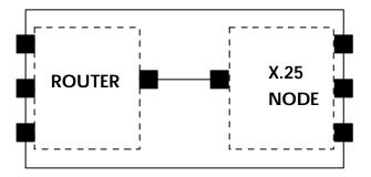
As can be seen in the figure, each virtual device manages its own set of interfaces.
