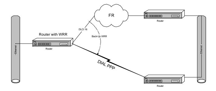
While the primary link is active, the secondary interface is on 'standby' i.e. as if it were down. If the RIP is enabled in the secondary link, calls are not provoked as the link is down. The traffic is routed through the primary link.
