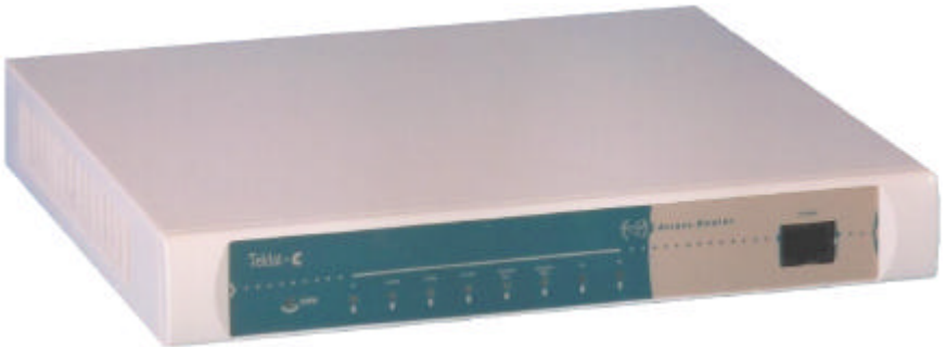
Illustration 1.1: External aspect for the Teldat C/S/G routers (excepting C6)
